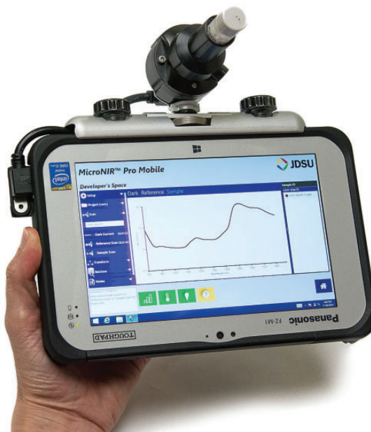
Figure 1. MicroNIR spectrometer equipped with a vial holder and tethered to a rugged 7" Windows 8.1 tablet for pharmaceutical raw material identification.
